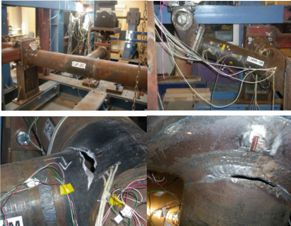
Figure 3.41. Pipe tee branches subjected to out-of-plane cyclic loading
