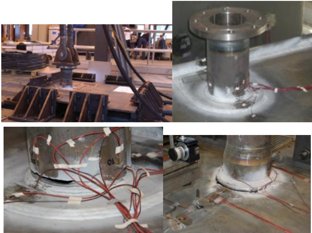
Figure 3.38. Mechanical behaviour of nozzles under strong repeated loading
