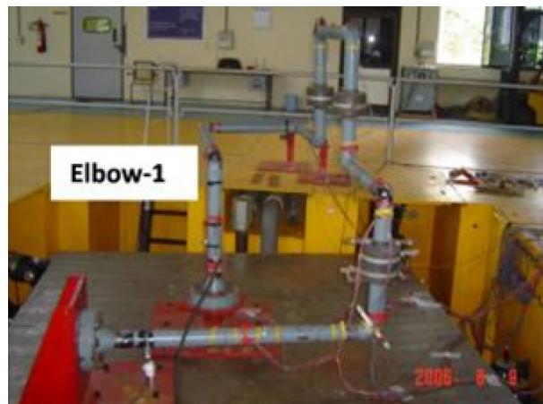
Figure 3.26. Photograph of the test setup of a three-inch CS piping system (CSPS3-1)
