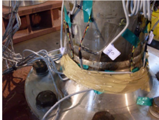
Figure 3.32. Photograph of weld failure at the anchor location in the SSPS-2 test
