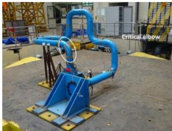
Figure 3.37. Photograph of the test setup of a six-inch CS piping system (schedule 80)
