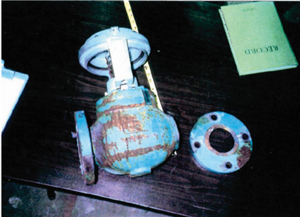
Figure B.12. View of a broken cast iron valve caused by the Northridge earthquake
