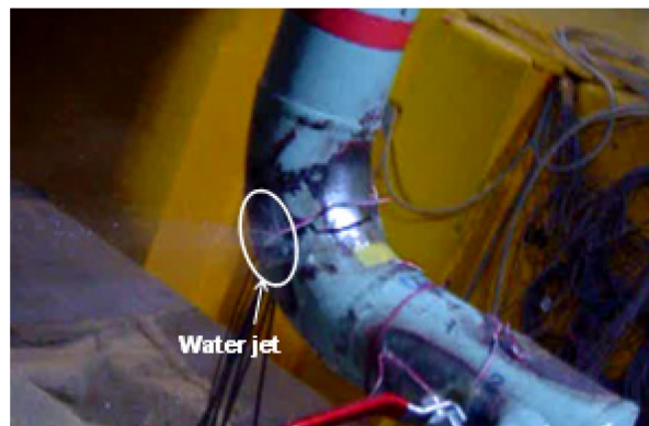
Figure 3.22. Photograph of fatigue-ratcheting failure at the crown location of a three-inch CS elbow
