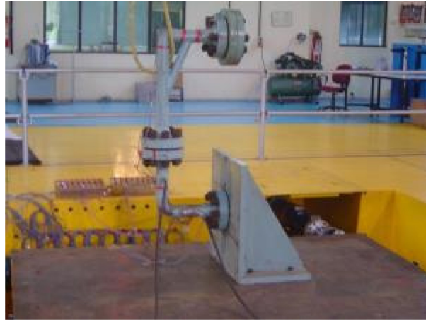
Figure 3.20. Photograph of the test setup of a three-inch CS elbow
