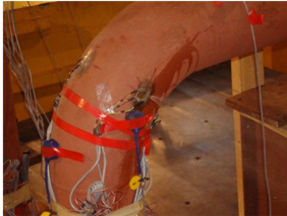
Figure 3.35. Photograph of fatigue-ratcheting failure at the crown of elbow-1 in the CSPA-1 test
