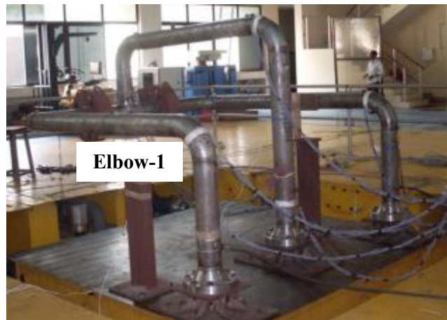
Figure 3.29. Photograph of the test setup of a six-inch SS piping system (SSPS-1)
