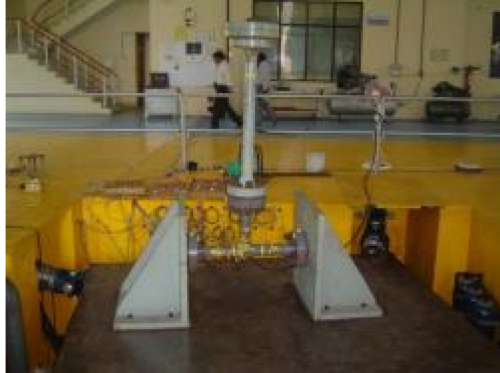
Figure 3.23. Photograph of the test setup of a three-inch CS Tee joint
