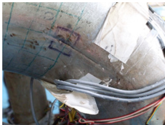
Figure 3.31. Photograph of a fatigue-ratcheting failure at the crown of elbow-1 in SSPS-1 test
